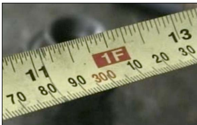
Figure 1. The marking lines to the left of one foot indicate fractions to thirty-seconds of an inch. On the right side of one foot the markings indicate fractions to sixteenths of an inch. (C has inscribed a line across the measuring tape with his pencil at 11 \frac{1}{8} "', partly obscuring the measuring tape inscriptions, and another short line over the marking at 11 \frac{5}{32} ".)
