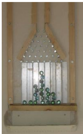
Figure 2 - Photo of our home-made Galton board
